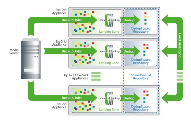
ExaGrid disk backup appliances include scalable computing software, which allows them to virtualize and share data storage capacity with one another. This scalable system (shown above) can expand as data grows by adding appliances, providing up to 4.6PB raw capacity, 4PB usable capacity, and allowing full backups of up to 2PB in a single scale-out system. Multiple systems can be used at a single location, and up to 16 separate locations can be managed through a single user interface.
