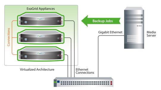
**ExaGrid Appliances Connect to Form a Single Scale-Out System**
