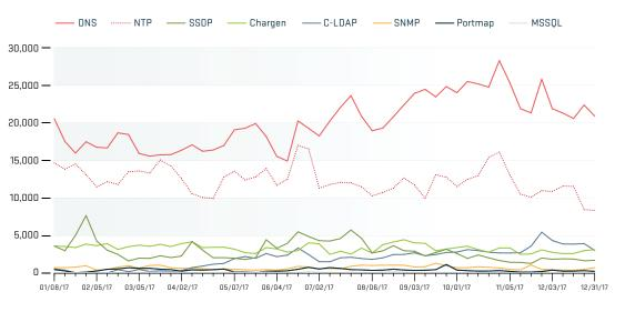
In 2016, we observed a resurgence of DNS as the dominant protocol used for reflection/ amplification attacks. This year, DNS continued to be the most common reflection/amplification attack vector. In fact, the number of DNS reflection/amplification attacks is greater than all the other attack vectors combined. The number of DNS attacks is nearly double the number of NTP reflection/amplification attacks, which came in second (Figure AT13).
