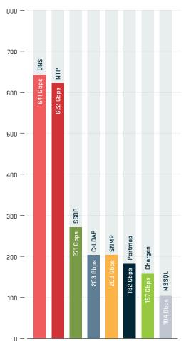
*Figure AT19 Reflection/Amplification Attacks, Peak Attack Sizes (Gbps)*
