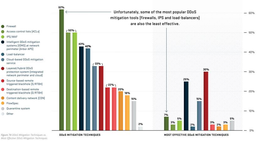
As in previous years, firewalls, IPS, WAF and access control lists (ACLS) remained the most common DDoS mitigation mechanisms for more than half of the respondents (Figure 74). The use of firewalls, IPS and WAF remains a concern as those devices are susceptible to state-exhaustion attacks, which were experienced by over a half of respondents.
